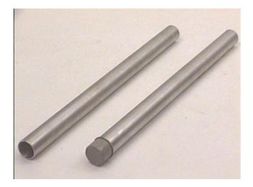
In fact, the frequency of the closed tube is approximately one octave - a factor of two in frequency - below that of the open tube.
