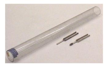
In fact, the frequency of the tube is one octave lower - a factor of two in frequency. The tuning fork is activating the second harmonic of the tube - twice its lowest resonant frequency.
