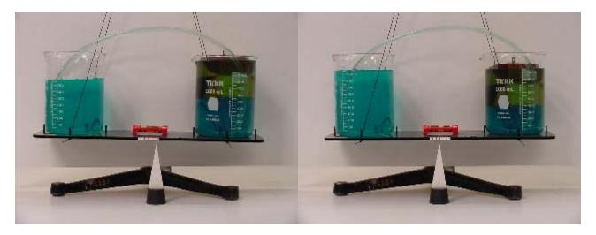
As in the previous examples, when the wood was placed into the beaker, the water level on that side rose, so the action of the siphon caused the system to equalize.
