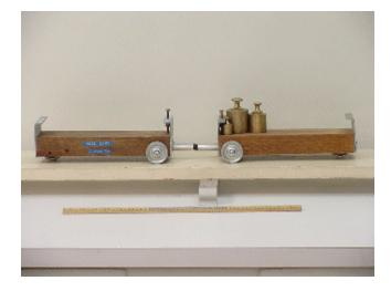
Because the mass of the cart on the right is twice that of the cart on the left, the cart on the right will leave the "collision" with half the velocity of the cart on the left. Therefore the beam will remain in balance until the lighter cart hits the end, after which time the board will tilt down to the right.
