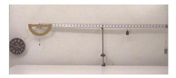
A greater force is required when it is applied at an angle because only the component of force perpendicular to the beam is relevant in producing torque. Here the applied force is about 14 Newtons at an angle of about  $45^{\circ}$ , so the downward component of this force is 14 Newtons x  $\cos(45^{\circ}) = 14$  Newtons x 0.7, approximately 9.8 Newtons, close to the value of 10.5 Newtons required when pulling straight downward.
