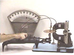
In this case the free electrons are moving through the magnet from the rear toward the front of the photograph, so, by the left hand rule for electrons, the fingers of the left hand point toward the right front of the photograph (the direction of electron motion) and curl *down* in the direction of the magnetic field (N to S), leaving the thumb pointing in the inward direction, the direction of the force on the electrons. The center of the disc is therefore more negative than the outside.
