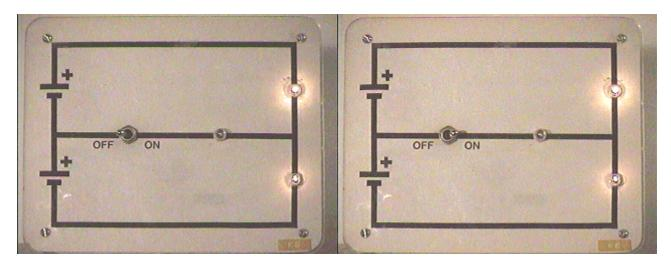
The center bulb will remain OFF. Because the two sides of the circuit connected by the middle wire are at the same potential, no current can flow in that wire, and the bulb will not be lit.
