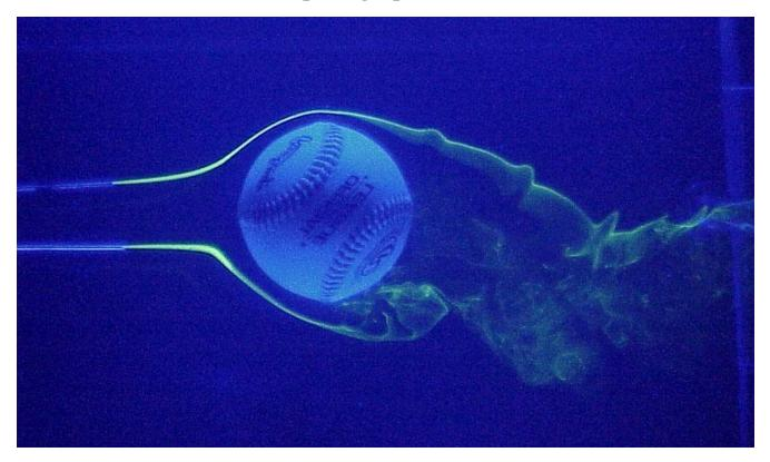
This picture is a view *looking downward* from above the ball, with the ball spinning clockwise as it moves from right to left across your computer screen, shedding vortices toward the bottom of the photograph so as to curve toward the top of the photograph. (A right-handed pitcher would achieve this effect by throwing the pitch side-arm and letting the ball slip off the end of her fingers as she released it.)
