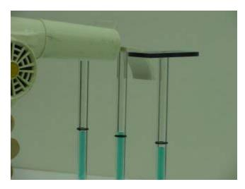
The answer to Part 3 is (c): the water level in the tube with the flat flange will remain the same, as can be seen in an mpeg video by clicking your mouse on the picture below.
