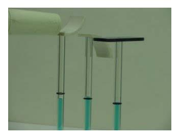
The answer to Part 2 is (a): the water level in the tube with the convex flange will go up, as can be seen in an mpeg video by clicking your mouse on the picture below.
