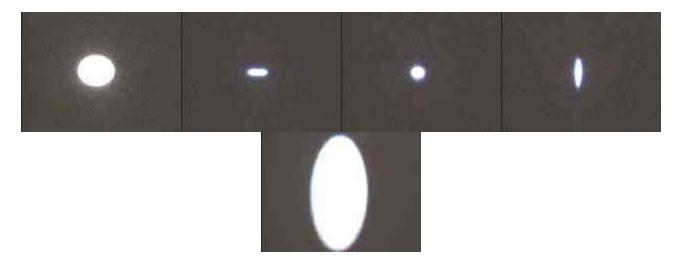
Note that because the vertical focusing is greater than the horizontal focusing the beam focuses in the vertical direction first, forming a horizontal line. The vertical line at the horizontal focus is longer because it is further from the astigmatic lens. The "average" focus, called the circle of least confusion, is not really a focus.
