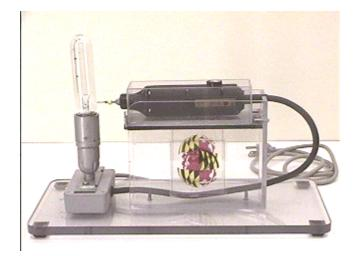
When air enters the bulb, the oxygen allows the filament to "burn" very strongly, so it burns up very quickly (within less than a second).
