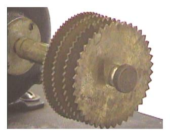
The number of teeth in the wheels, right to left, is in the ration 4:5:6:8, which is the frequency ratio of the notes in a major chord, such as the 4<sup>th</sup>, 5<sup>th</sup>, 6<sup>th</sup>, and 8<sup>th</sup> harmonics of the overtone series, shown in the figure below.
