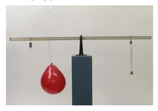
When the string is burned, the weight of the balloon is removed from the left side, leaving a net torque downward on the right side, so the right side will go down.
