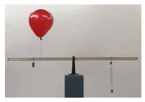
When the string is burned, the upward buoyant force of the balloon is removed from the left side, leaving a net torque downward on the left side, so the left side will go down.
