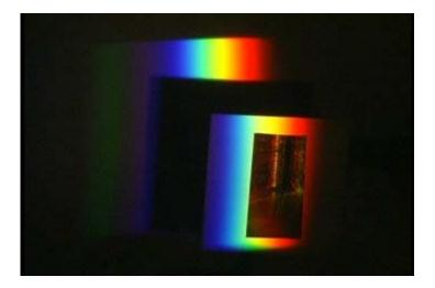
Although blue (and green as well as every other color) photons are more energetic than red photons, the frequency will decrease, because the thermopile is sensitive to *infrared* photons. This is a *heat-sensing* device, as demonstrated using <u>Dan's head</u> in Question #247.
