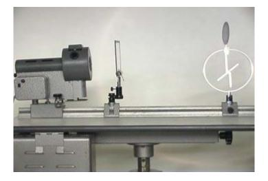
The UV photons are totally absorbed by single electrons in the negatively charged zinc plate, giving the electron enough energy to leave the plate. In this case they possess enough kinetic energy to allow them to escape from the plate entirely, reducing the negative charge level on the plate. Further, the negative charge on the plates provides additional repulsion of the escaping electrons.
