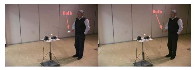
The waves from the transmitting antenna are polarized in the horizontal direction - the orientation of the antenna. A receiving antenna perpendicular to the receiving antenna will only send or receive vertically polarized waves, so the light will go out.
