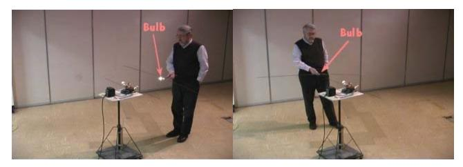
The waves from the transmitting antenna form a "dipole antenna pattern" in the horizontal plane with the maximum energy flowing away from the center of the antenna in a plane perpendicular to the antenna. There is a minimum of energy flow along the line of the antenna. This means that the "antenna pattern" of radio or TV stations may affect the direction in which the signal is larger or smaller, or may even result in the signal being so small that a station cannot be received.
