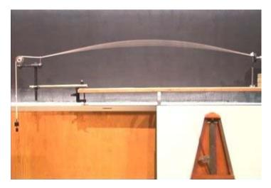
If this video goes by too fast, click your mouse <u>here</u> to see a slow-motion version. Note that for the first part (the two-loop standing wave) there are four wave vibrations per metronome tick, while after the frequency has been changed (the single loop standing wave) there are two wave vibrations per metronome tick. Reducing the frequency by a factor of two increases the wavelength by a factor of two, so the length of the vibrating rope includes a single loop rather than two loops.
