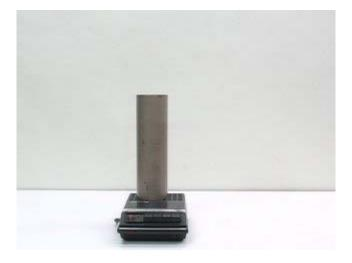
The resonance of the tube enhances frequencies near the resonant frequency of the tube. The tube functions as an open tube of length about 64 cm (including the end correction for the top end), which is about 540 Hz. The sound of the noise persists, however, because the tube does not have a very high Q (resonant quality factor) and because noise frequencies over a large range of the audible frequency band are present with significant amplitudes.
