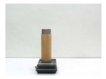
When the tube becomes longer, the wavelength increases, causing the pitch to decrease.
