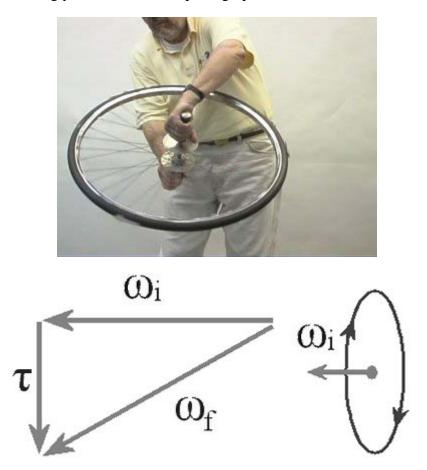
Note that in this case the vector angular momentum originally points toward your left as you view the spinning wheel. When you rotate the wheel counterclockwise as viewed from above, you exert a vector torque in the **downward** direction. Therefore the angular momentum change must be in the downward direction, leading to a net angular momentum that is pointed to the left but slightly in the downward direction, as seen in the photograph and in the drawing at the right.
