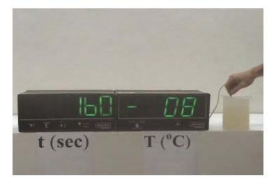
As time goes on and the salt is continually mixed into the icewater, the video has been edited to show short segments of the action such that you can see the temperature of the mixture as a function of time.
