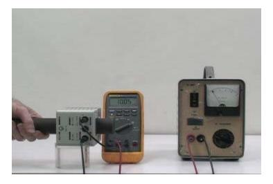
In order to conserve energy in the magnetic field, as the core is removed the current must rise. Equivalently, as the core is withdrawn the collapsing magnetic field in the coil induces a current in the same direction as the current provided by the power supply, according to Lenz's law. The current therefore rises, but rapidly returns to its original value due to the resistance of the coil.
