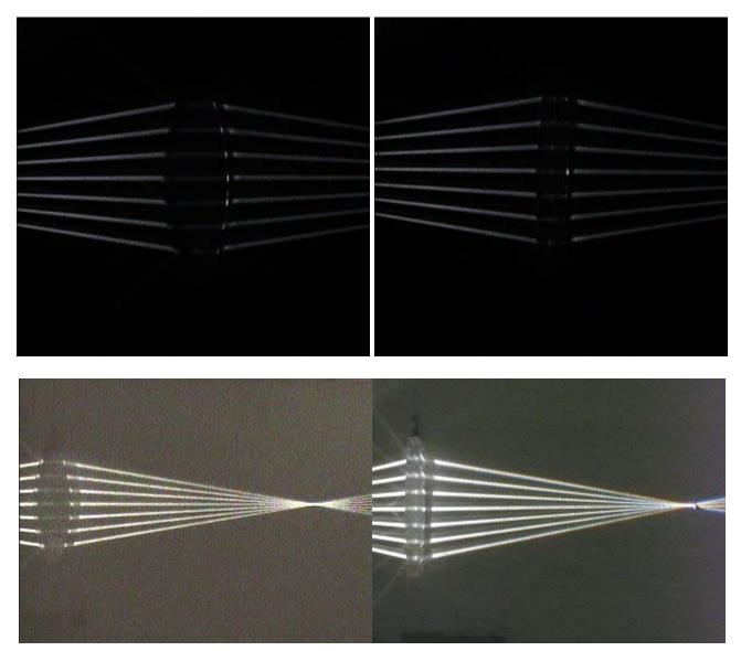
The refraction of a lens occurs when the light *enters* or *exits* the lens, and no bending of the light occurs as the light travels *through* the lens. Because the entrance and exit angles of the original lens and the equivalent Fresnel lens are identical for a light ray entering the lens at the same distance from the optic axis, the focal properties of the two lenses will be virtually identical.
