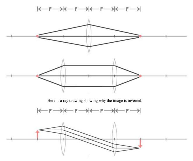
Notice that the optical arrangement is symmetrical; the existence of this symmetry is also a clue as to the location and the inversion of the image.
