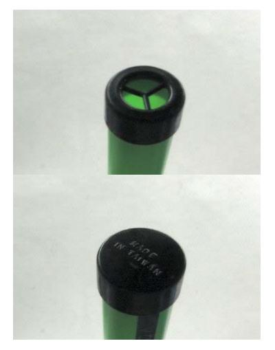
This is a model of formants in the human voice. The reed vibrates at a certain frequency as air rushes through it, creating a fundamental with a large number of overtones. As the length of the tube increases, its resonant frequencies become lower, so it sounds more like a vocal "oo." As the length of the tube decreases, its resonant frequencies become higher, so it sounds more like a vocal "ah."
