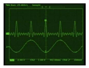
Note that if all of the *odd* harmonics are removed, the remaining harmonics are 2, 4, 6, 8, etc; this is just the same overtones as a note whose fundamental frequency is twice that of the original note, including all harmonics with the same amplitudes and the same phase relationship.
