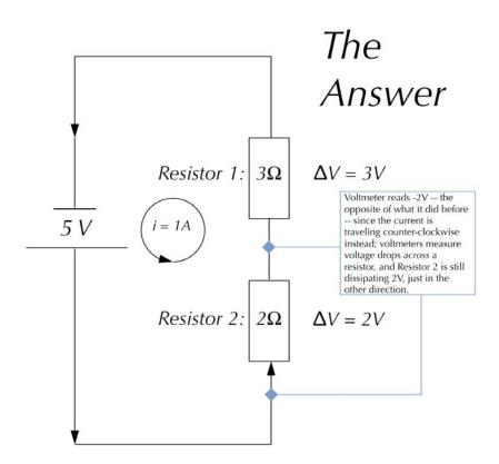
While the argument for option (b) is quite plausible -- that the voltage will drop across Resistor 2 first, and therefore the meter reads 3V -- one must keep in mind we aren't exactly measuring *the* voltage between the two resistors; we are measuring the difference in voltage *across* Resistor 2. By Ohm's law, we know Resistor 2 must dissipate 2V, and the magnitude of the voltmeter must be 2V. Whether it's positive or negative indicates it's a positive change or negative change.
