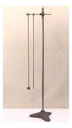
This is the location of the radius of gyration of the physical pendulum - the length of a simple pendulum with its period equal to that of the physical pendulum. Try comparing the periods of a physical pendulum and a simple pendulum with 2/3 the length of the physical pendulum.
