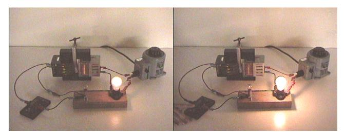
Even with no secondary current, the impedance of the primary coil is sufficiently low to draw enough primary current to light the primary light bulb. As seen in the photograph at the right, the secondary bulb is just barely glowing, but this requires enough additional current in the primary to make the primary bulb glow significantly more brightly.
