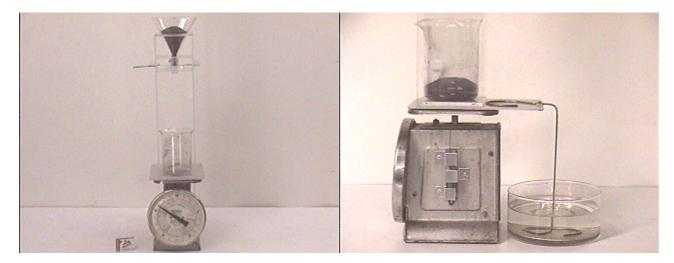
The photograph at the right shows the setup from the side. A metal plate attached to the surface of the scale and extending into a water bath serves as a damping device to limit the excursion and oscillation of the scale after a rapid change occurs. You may notice from the video that we are actually using small lead shot in place of sand to enhance any effects.
