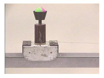
The ball falls BEHIND the funnel because the cart is being accelerated. After the ball is ejected its horizontal velocity remains constant, while the horizontal velocity of the cart continues to increase, so the cart accelerates away from the ball.
