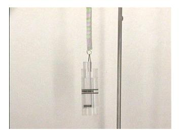
This happens for the same reason that the floater remains at the same position in the water bath as the water container oscillates. Even when the motion is stopped short the ratio of weight density between the water bath and the floater remains constant!
