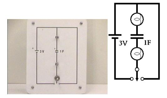
When the switch is closed, current begins to flow through the entire circuit, lighting both lamps. As the capacitor becomes charged, the current reduces exponentially to zero, when the capacitor is fully charged and the light bulbs cease to glow.
