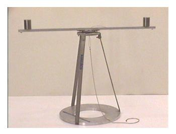
This is due to conservation of angular momentum. The angular momentum of the system L = mvr, where m is the mass of the rotating weights, r is their radius, and v is their speed (neglecting the mass of the crossarm). When the wires pull the masses in, no torque is exerted on the system so its angular momentum remains constant. Because the radius of the masses decreases, their speed must increase.
