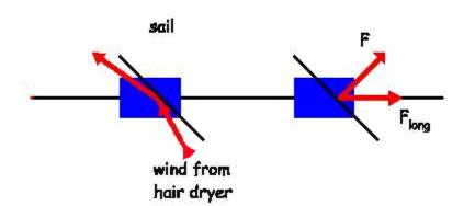
When the air stream deflects off the sail, it sets exerts a force vector as seen in the diagram at the right above. Because the glider can only move along the air track, the component to the right in the diagram causes the glider to move to the right.
