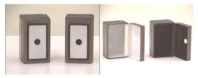
These boxes are examples of blackbody radiation: the spectrum of the radiation emerging from the holes is a function only of the temperature, which is the same for both boxes. Therefore the color of both holes is the same.
