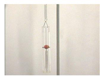
This device is a type of accelerometer, in which the pingpong ball moves in the direction of the acceleration at each point in the motion of the container. Thus, when the container is above its equilibrium position the acceleration is downward, but when the container is below its equilibrium position the acceleration is upward.
