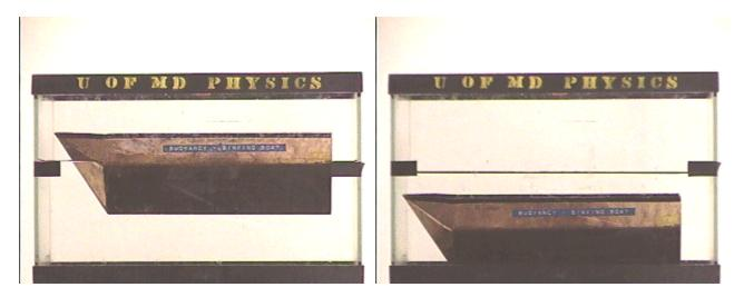
This problem is essentially the same as <u>Question 17</u>. When the boat is floating, it displaces its weight in water. After the boat has sunk, it displaces its volume in water, which is much less water, so the water level in the pond goes down.
