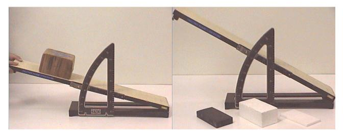
Now suppose that the experiment is repeated using the blocks seen in the photograph at the right above: rubber, styrofoam, and teflon (alphabetically, left to right). Which will begin to slide first and which last when the tilt of the incline is increased?
