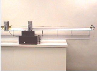
Releasing *M* allows *m* to accelerate it along the air track. The timer measures the time taken for a flag on the top of the air track glider to travel from photocell gate "A" to gate "B," which turns out to be exactly 2.00 seconds. See a video of the action by clicking your mouse on the photograph above.
