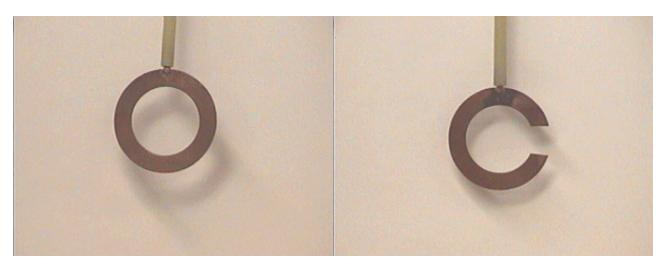
Question: Which of these bobs will be damped out more rapidly and which less rapidly when they are lifted to a horizontal position and released?
