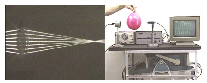
The same experiment can be performed with sound using a balloon as a "sound lens," because the shape of an inflated balloon is similar to that of a light lens. The experimental arrangement is shown in the photograph at the right above. Sound from the microphone, at the left of the balloon, is focussed by the balloon onto the microphone, at the right of the balloon.
