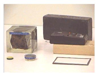
If something is placed between the radioactive source and the detector, the particles might be stopped. The photograph also shows three possible "stoppers" of nuclear radiation: a lead brick, a thin sheet of lead, and a piece of paper (on the lead sheet).
