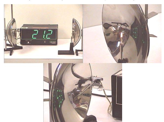
When the match is lit, as shown in the photograph at the left below, infrared radiation from the flame is reflected by the mirror at the right into a parallel beam, then focused by the mirror at the left onto the thermal probe. This causes the temperature to rise to 23.7° C, as seen in the photograph. This temperature took a couple of minutes and a couple of matches, but virtually any type of small heat source will work.
