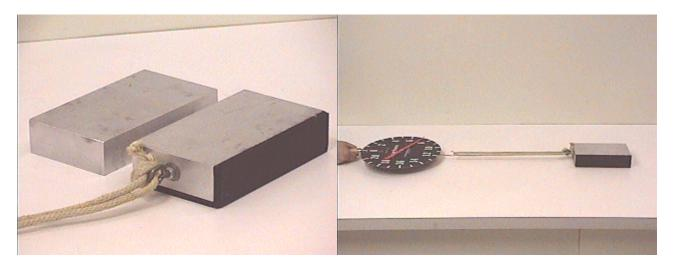
Now suppose the you turn the block onto its smaller surface, which is also covered with the same type of rubber, and pull it the same way with the spring scale.
