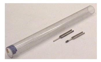
In this case the tube is about 68 cm long and about 6 cm in diameter, the frequency of the tuning fork is 480 Hz, and the speed of sound is approximately 345 m/s. When you blow across the end of the plastic tube you can create a musical tone. We now wish to compare the frequency of the tuning bar with that obtained by blowing across the end of the tube.
