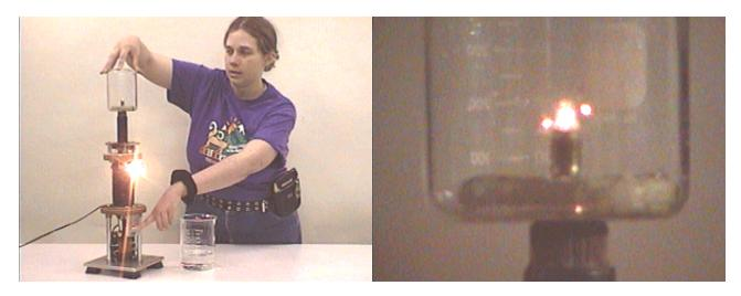
Gwen is holding a beaker in which a small coil with a light attached to it has been placed, as seen in the photograph at the right. The changing magnetic field, exiting the magnetic core of the Thomson coil and passing through the small coil, induces an electrical potential in the coil that lights the lamp. The question this week regards what will happen to the light when water is poured into the beaker, covering the coil and the light bulb.
