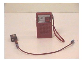
Gwen is going to hold a 9-volt battery, seen in the photograph, near the radio and use the attached clip lead to short out the battery, connecting and disconnecting the wire across the battery terminals. The question is what, if any, effect will be heard on the radio.
